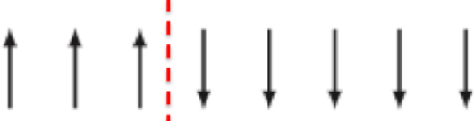
FIG. 4: The creation of a domain wall in one dimension. Domain wall is indicated in red [4].
