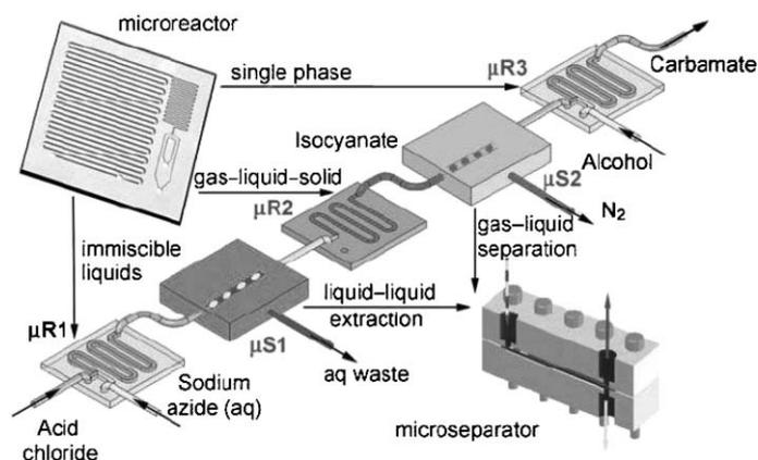
**Fig. 2** Microfluidic device for the multistep carbamate synthesis. The process involves three reaction steps, conducted in the modules  $\mu R1$ ,  $\mu R2$  and  $\mu R3$ , and two separation steps, performed in the modules  $\mu S1$  and  $\mu S2$ . (Adapted with permission from Sahoo *et al.*<sup>3</sup> Copyright 2007, Wiley-VCH.)
