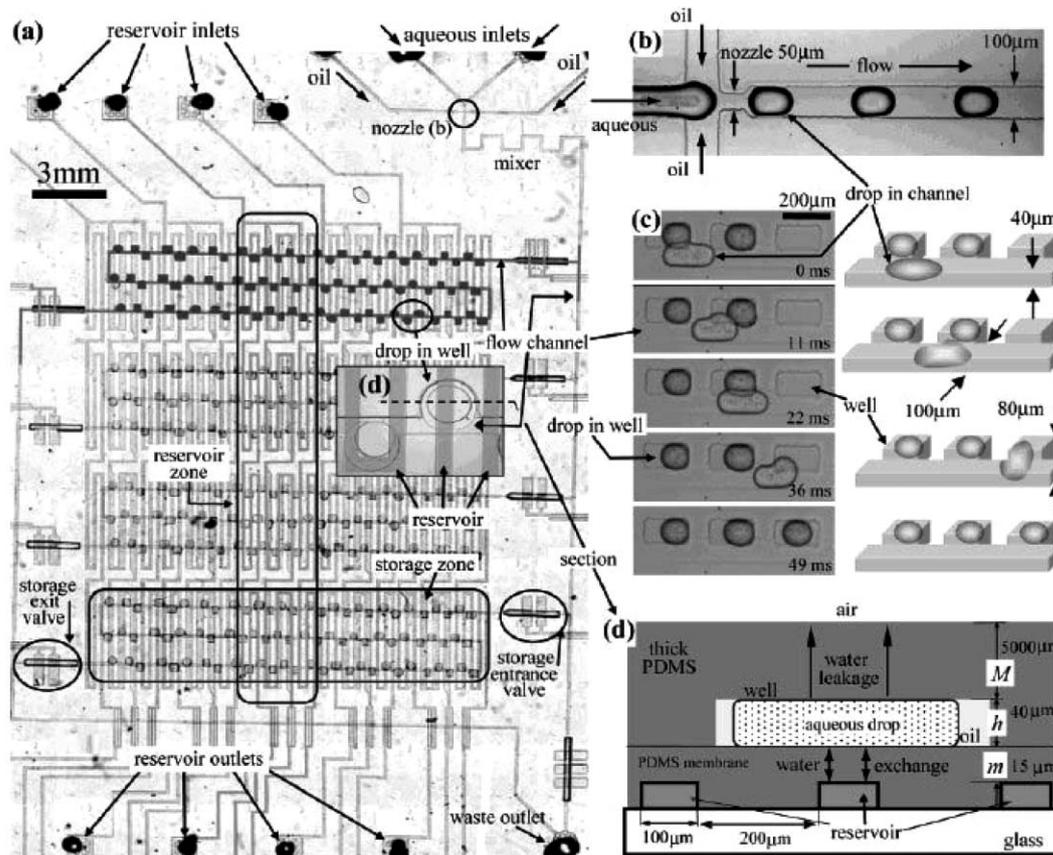
**Fig. 1** (a) Design of the microfluidic device (“Phase Chip”) to determine the phase diagram of multicomponent fluid mixtures in micro-sized droplets. (b) Droplets are formed by hydrodynamic focusing of an aqueous solution into two streams of hydrophobic carrier fluid (oil). (c) Surface tension guided storage of droplets into wells. (d) Vertical section of the storage wells. (Reprinted from Shim *et al.*<sup>2</sup> Copyright 2007 American Chemical Society.)
