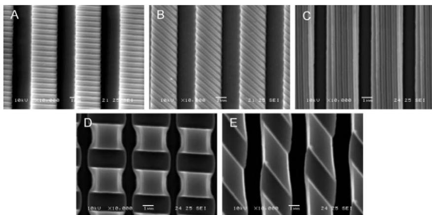
**Fig. 3** Tunable anisotropic wettability on polymer surfaces. The figure shows SEM images of polymer films with two-level hierarchical structures that consist of micrometre and submicrometre scale gratings. (Reprinted from Zhang and Low.<sup>4</sup> Copyright 2007 American Chemical Society.)
