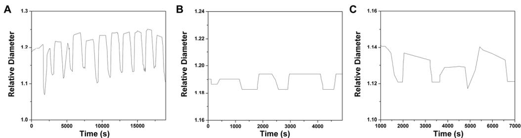
**Figure S9.** Oscillating volume change profile of Gel<sub>c</sub> under the flow of BZ solution (10  $\mu\text{L}/\text{min}$ ,  $[\text{NaBrO}_3] = 0.2 \text{ M}$ ,  $[\text{CH}_2(\text{COOH})_2] = 0.4 \text{ M}$ , and  $[\text{HNO}_3] = 0.4 \text{ M}$ ) at 10 °C (A), 14 °C (B) and 18 °C (C).
