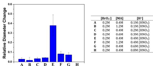
**Figure S6.** The relative volume change of the oscillating Gel<sub>a</sub> at same continuous-flow rate (10 μL/min) in the same microfluidic channel but different BZ reactant (listed in the table) at 10 °C.
