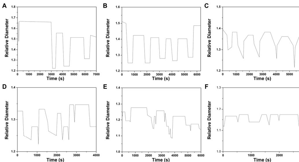
**Figure S7.** Oscillating volume change profile of Gel<sub>a</sub> under a flow of BZ solution (10 μL/min, [NaBrO<sub>3</sub>] = 0.2 M, [CH<sub>2</sub>(COOH)<sub>2</sub>] = 0.4 M, and [HNO<sub>3</sub>] = 0.4 M) at (A) 10 °C, (B) 14 °C, (C) 18 °C, (D) 22 °C, (E) 26 °C and (F) 30 °C.
