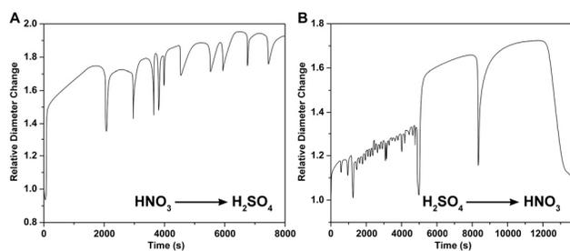
**Figure S12.** Relative volume change profiles of  $Gel_a$  at same continuous-flow rate ( $10 \mu\text{L}/\text{min}$ ) but with counter ion exchange (A) from  $\text{HNO}_3$  to  $\text{H}_2\text{SO}_4$  and (B) from  $\text{H}_2\text{SO}_4$  to  $\text{HNO}_3$ .
