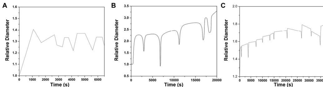
**Figure S8.** Oscillating volume change profile of  $\text{Gel}_b$  under a flow of BZ solution ( $10 \mu\text{L}/\text{min}$ ,  $[\text{NaBrO}_3] = 0.2 \text{ M}$ ,  $[\text{CH}_2(\text{COOH})_2] = 0.4 \text{ M}$ , and  $[\text{HNO}_3] = 0.4 \text{ M}$ ) at (A)  $14^\circ\text{C}$ , (B)  $22^\circ\text{C}$  and (C)  $30^\circ\text{C}$ .
