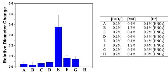
**Figure S6.** The relative volume change of the oscillating  $\text{Gel}_a$  at same continuous-flow rate ( $10 \mu\text{L}/\text{min}$ ) in the same microfluidic channel but different BZ reactant (listed in the table) at  $10^\circ\text{C}$ .
