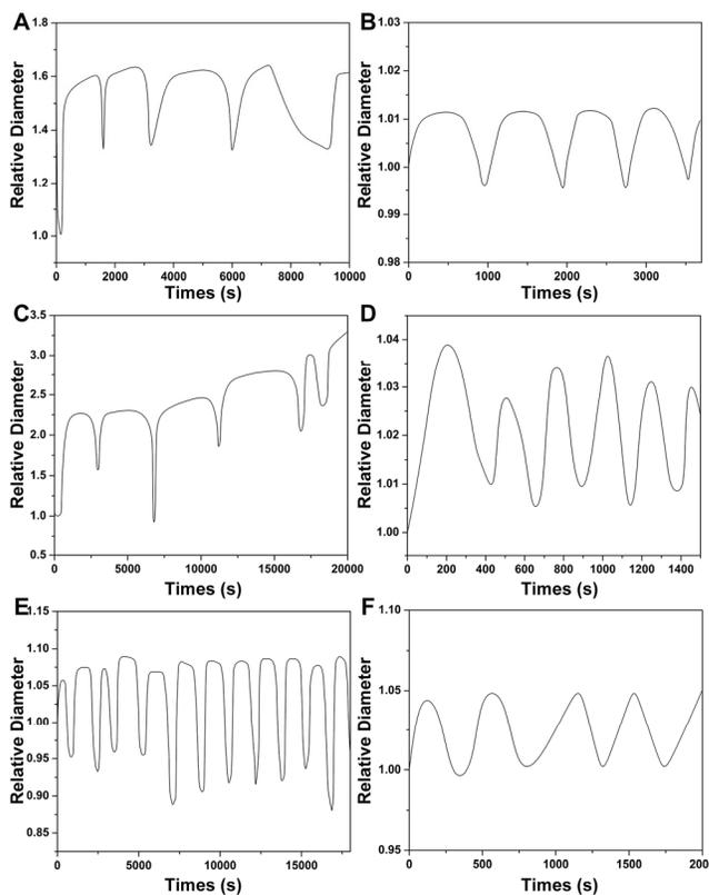
**Figure S10.** Oscillating volume change profiles of (A) Gel<sub>a</sub>, (C) Gel<sub>b</sub> and (E) Gel<sub>c</sub> with continuous flow, (B) Gel<sub>a</sub>, (D) Gel<sub>b</sub> and (F) Gel<sub>c</sub> without flow under optimal BZ conditions.
