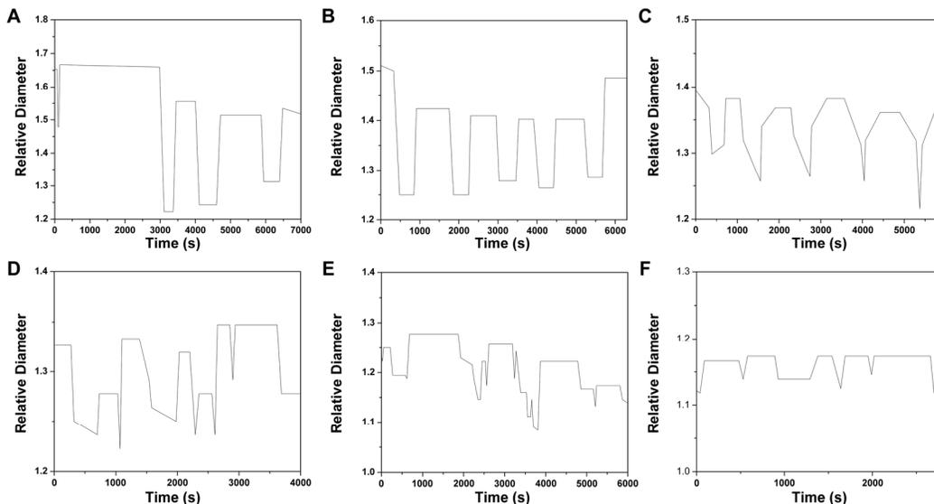
**Figure S7.** Oscillating volume change profile of  $\text{Gel}_a$  under a flow of BZ solution ( $10 \mu\text{L}/\text{min}$ ,  $[\text{NaBrO}_3] = 0.2 \text{ M}$ ,  $[\text{CH}_2(\text{COOH})_2] = 0.4 \text{ M}$ , and  $[\text{HNO}_3] = 0.4 \text{ M}$ ) at (A)  $10^\circ\text{C}$ , (B)  $14^\circ\text{C}$ , (C)  $18^\circ\text{C}$ , (D)  $22^\circ\text{C}$ , (E)  $26^\circ\text{C}$  and (F)  $30^\circ\text{C}$ .
