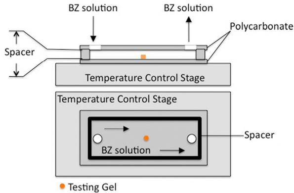
**Figure S5.** Cartoon illustration of the set-up of the microfluidic flow cell for detection of chemomechanical oscillation of the microgels under a bright field microscope and on a temperature control stage.
