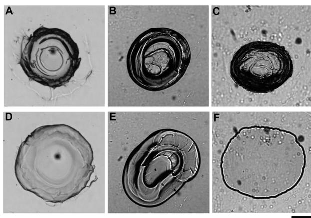
**Figure S4.** Optical images of gels in the reduced state before and after several hours of BZ reaction. Gel<sub>a</sub> at (A) 0 and (D) 6 h of BZ oscillation; Gel<sub>b</sub> at (B) 0 and (E) 4 h of BZ oscillation; Gel<sub>c</sub> at (C) 0 and (F) 6 h of BZ oscillation (scale bar is 100  $\mu\text{m}$ ).
