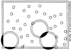
Walls and big balls create zones (light blue) where room to roam is lost by some part of each small ball. For instance, a small ball's center is stopped a full radius (r) away, whereas points on its surface roam everywhere. To increase room to move, or entropy, small balls herd large ones into the corners and against the walls and each other. Where surfaces of large balls and walls touch, the restricted regions overlap (dark blue), freeing unfettered volume elsewhere.
